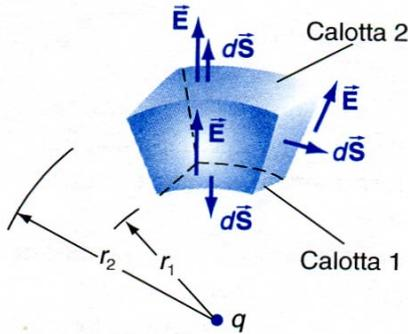
$$\begin{aligned} \Phi_1 &= \oiint_{S_1} \vec{E} \cdot d\vec{S} = \iint_{S_1} -E dS = \iint_{S_1} -\frac{q}{4\pi\epsilon_0 r_1^2} dS = \\ &= -\frac{q}{4\pi\epsilon_0 r_1^2} \iint_{S_1} dS = -\frac{q}{4\pi\epsilon_0 r_1^2} \Delta S_1 \end{aligned}$$
