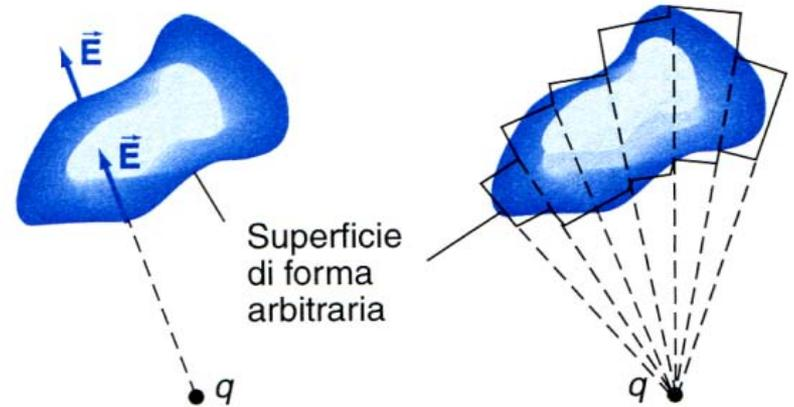
$$\begin{aligned}\Phi_E &= \oiint_{\text{Sfera}} \vec{E} \cdot d\vec{S} = \iint_{\text{Sfera}} E_r dS = E_r \iint_{\text{Sfera}} dS = \\ &= \frac{q}{4\pi\epsilon_0 r^2} 4\pi r^2 = \frac{q}{\epsilon_0}\end{aligned}$$
